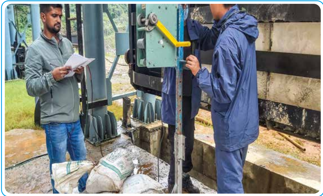
Flow measurement at tailrace of Mистри Khola HEP
