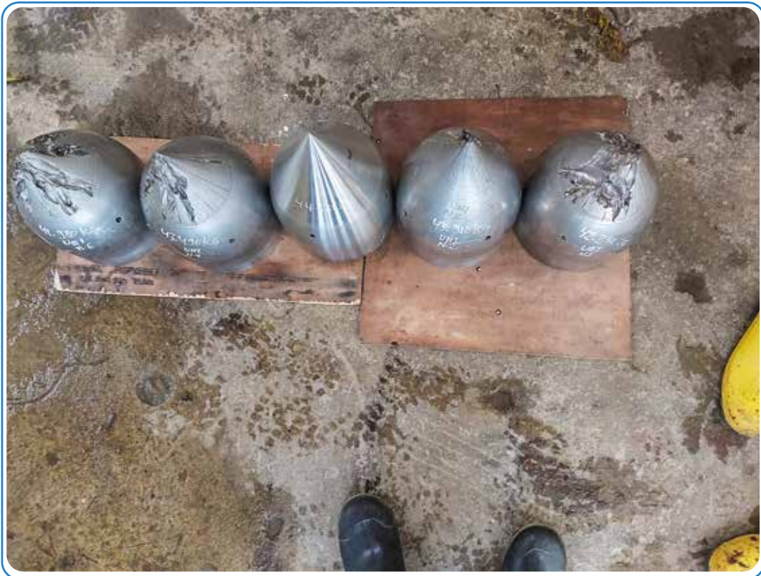
Eroded needle tips changed in 2080.06.04 in Unit#1 of Mistri Khola HEP
